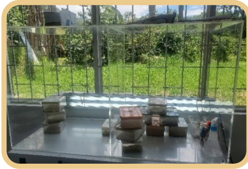
Figure 36. Acrylic chambers 90 cm long x 60 cm wide x 50 cm high with a horizontal LED lamp.
