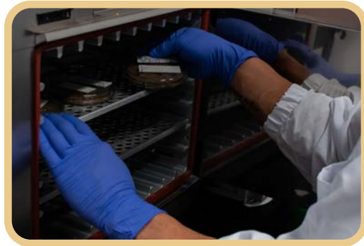
Figure 30. Phymastichus coffea artificial substrate drying process at 45-47°C.
