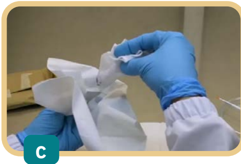
Figure 31. a. Disinfection of CBB in 0.5% sodium hypochlorite solution. b. Rinse three times with distilled water using a muslin cloth. c. Remove wet excess using a disposable towel.
