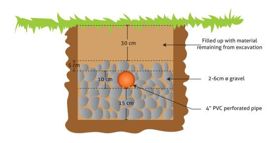
Figure 39. Diagram of one of the drain trenches. Source: colombit, 2000
