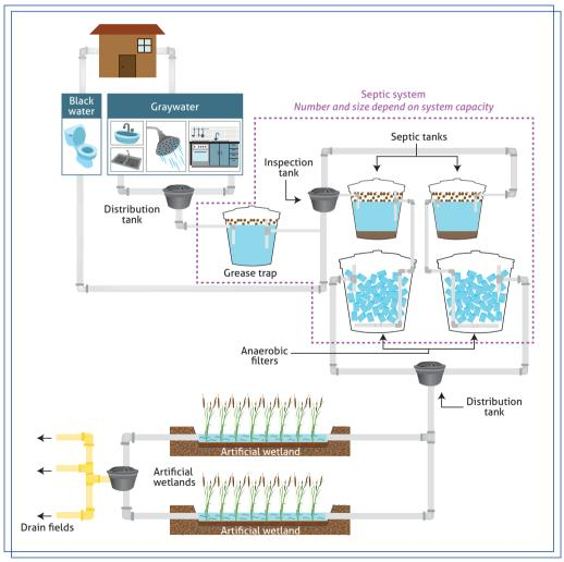
Figure 40. Integrated domestic wastewater treatment system diagram.
