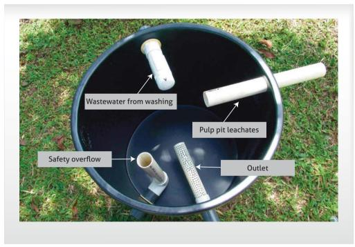
Figure 42. Pulp trap diagram.
