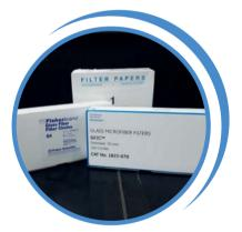
**Total Suspended Solids (TSS):** Nonfilterable residue or undissolved material present in wastewater (Figure 5).
