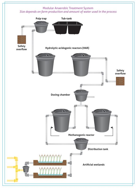
Figure 41. Modular Anaerobic Treatment System Diagram.
