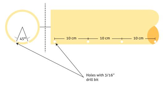
Figure 38. Diagram of holes in distribution pipes. Source: colombit, 2000
