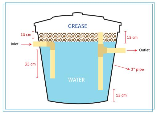
Figure 17. Grease trap.
