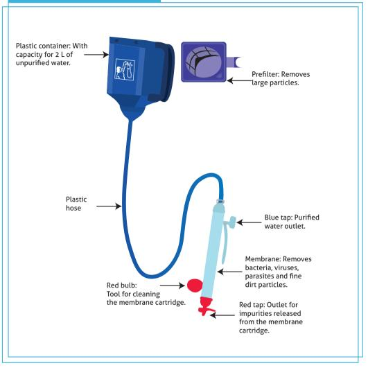
Figure 13. Nanofiltration system (Source: www.iwanagreen.com).
