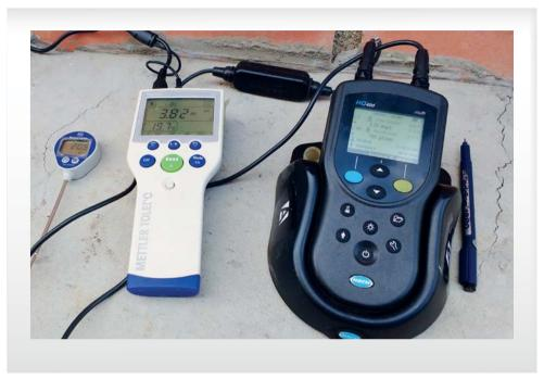
Figure 9. Equipment for determination of pH.
