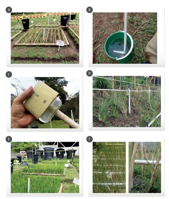
Figure 51. (a) The plots before the experiment; (b) Horizontal suction lysimeter; (c) Sampling container and irrigation system; (d) Leveling of irrigation pipes; (e) Plots at completion of the experiment; (f) Flow distribution system.
