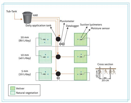
Figure 49. Diagram of experimental vegetation filter plots.
