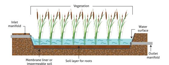
Figure 30. Free water surface wetland diagram (Source: EPA, 2000).
