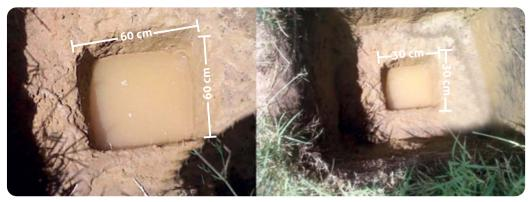
Figure 36. Percolation tests for design of drain fields.
