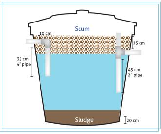
Figure 20. Details of septic tank.
