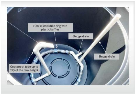
Figure 43. Hydrolytic-Acidogenic Reactor diagram.
