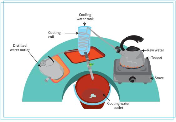
Figure 12. Distillation system with teapot.
