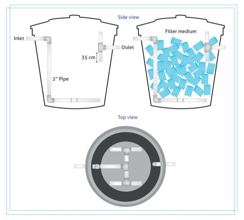
Figure 29. Characteristics of anaerobic filters.
