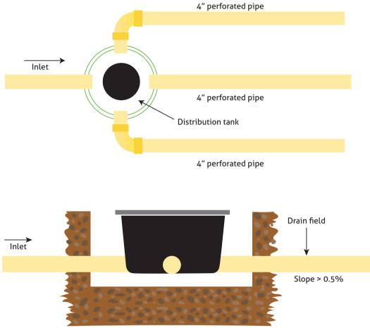
Figure 37. Distribution tank diagram. Source: colombit, 2000
