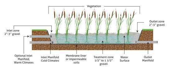
Figure 31. Constructed subsurface flow wetland diagram (Source: EPA, 2000).
