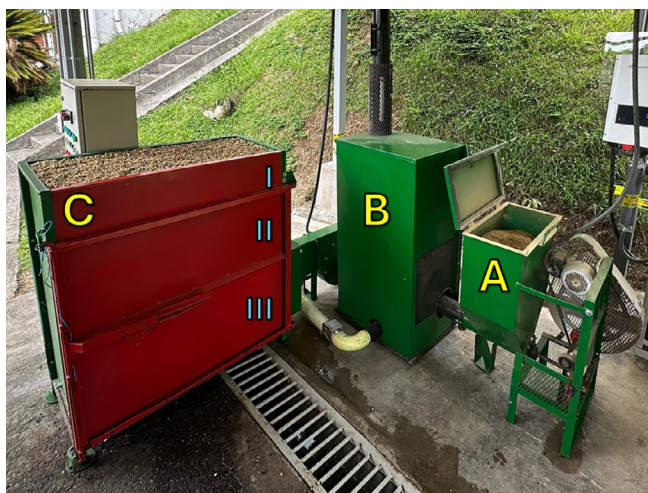
FIGURE 1 | Biomass heated convective dryer used for the experimental drying of Coffea arabica L. var. Cenicafé 1 parchment coffee. (A): Husk hopper, (B): Biomass burner and heat exchanger, (C): Drying chamber with three trays (I, II, III). Only the upper tray (I) was used during the tests.
