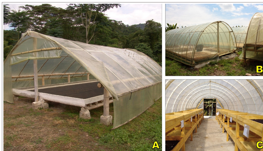
Figure 4. Different configurations of parabolic greenhouse-type solar dryers: (A) Low-profile parabolic dryer with raised concrete bed, (B) high-arched passive solar tunnels, and (C) internal view of a multi-tier greenhouse dryer illustrating vertical space utilization for batch drying.
