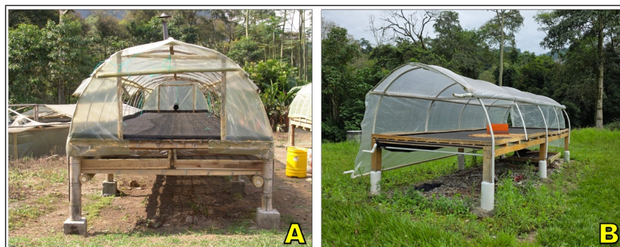
Figure 5. Comparative structural configurations of passive solar tunnel dryers for parchment coffee: (A) A sustainable framework constructed from Guadua angustifolia Kunth (structural bamboo) clad with UV-stabilized low-density polyethylene (LDPE) greenhouse-grade film; (B) a lightweight polyvinyl chloride (PVC) vaulted frame featuring woven poly-laminate (scrim-reinforced) fabric.
