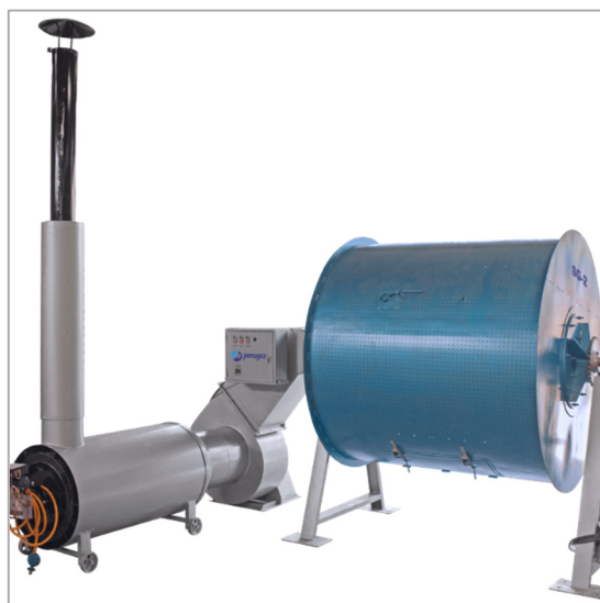
Figure 10. Industrial rotary drum dryer. Thermal energy generation unit featuring a chimney for combustion gas evacuation and a centrifugal fan for forced convection; a perforated rotary drum designed for batch or continuous operation. Penagos Hermanos. Coffee Processing Plants. Available online: https://penagos.com/centrales-de-procesamiento-de-cafe/ (accessed on 27 April 2026).
