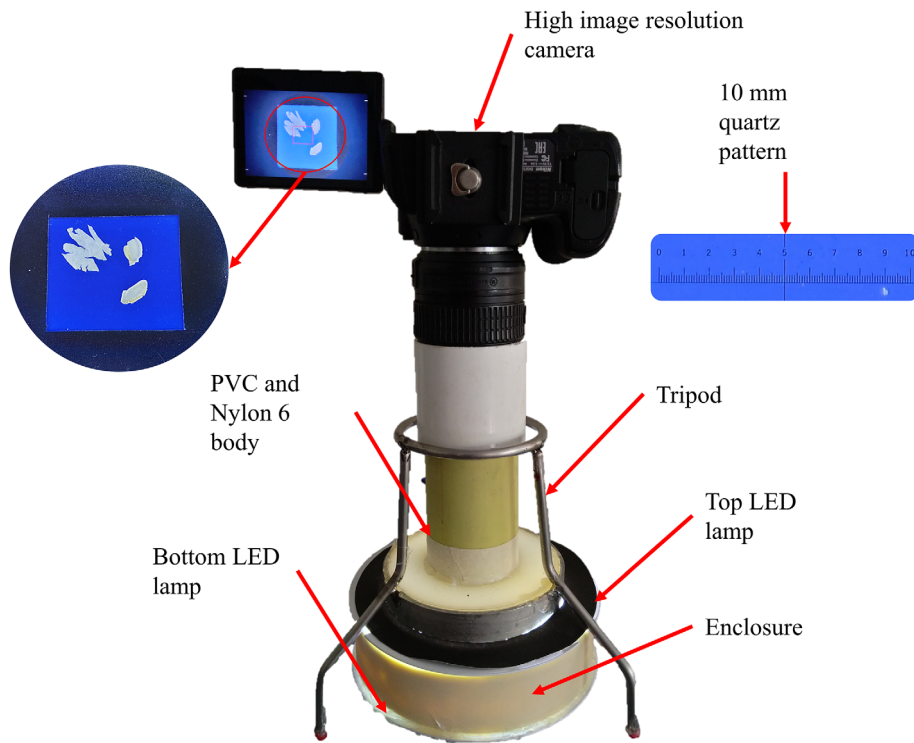
FIGURE 2 Coffee endocarp photographing setup.
